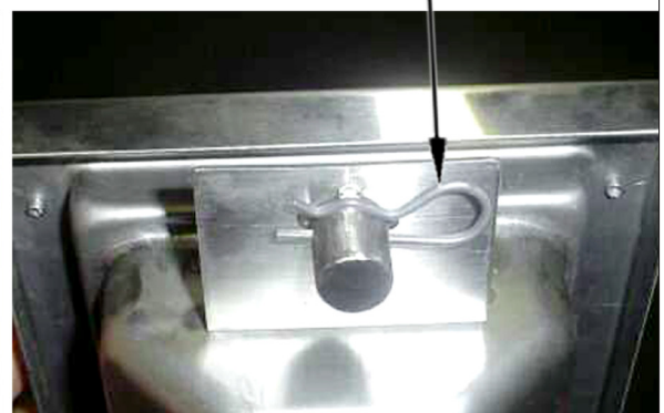
Locking pin on infrared burner
