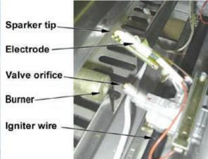
**Problem:** Burner tube is misaligned over the orifice
