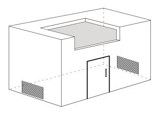
At least two ventilation openings at cylinder valve level shall be provided in the side wall, equally sized, spaced at 180 degrees and unobstructed.
